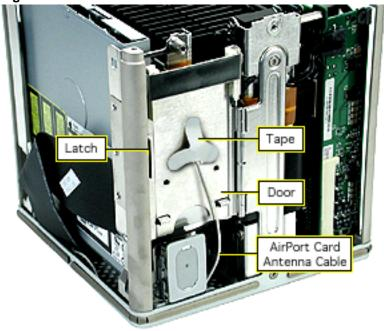
3. Using a magnetized screwdriver, remove the two screws from the side of the drive. Repeat on the other side. **(Figure 9)**
